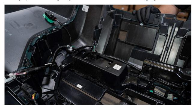
1.20 - Start by unplugging the fog light connector, then disconnect the front sensors to fully free up the components.
