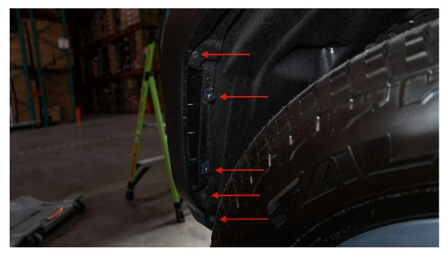
1.6 - Next, remove the six 10mm bolts shown in the image below.
