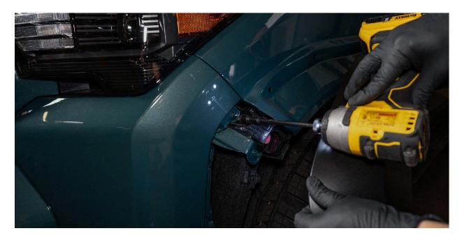
1.12 - Now, move to the front center section of the bumper. You'll find two 10mm bolts that need to be removed.
