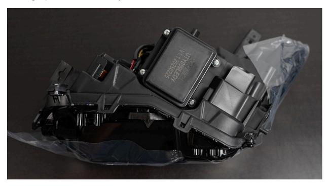
1.2 - Using a Phillips head screwdriver, carefully remove the four screws holding the control board in place.
