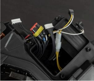
1.7 - Take your replacement control board and reconnect the six plugs into their corresponding ports.
