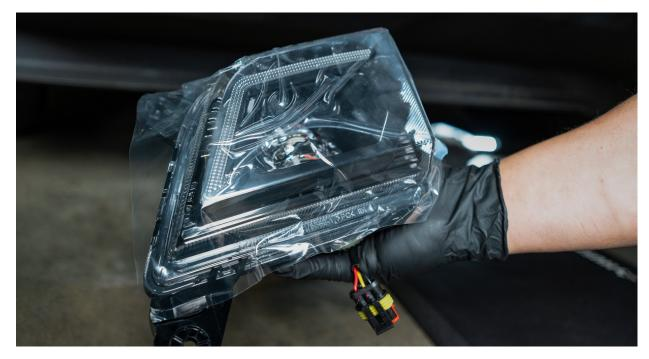
2.2 - When installing the Alpharex fog light, you'll notice it has two plugs instead of one. This is because our fog lights require a separate harness to power the DRLs and sequential turn signals.
