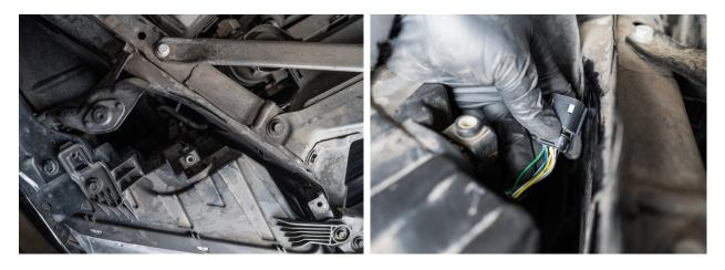
2.10 - Clip the yellow wires to the turn signal wires on both headlights (6th pin) and the red wire to the parking light (8th pin) on the driver's side.
