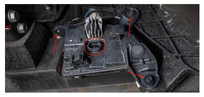
1.2 - Once all the bolts are removed and the plug is disconnected, the fog light can be easily removed.
