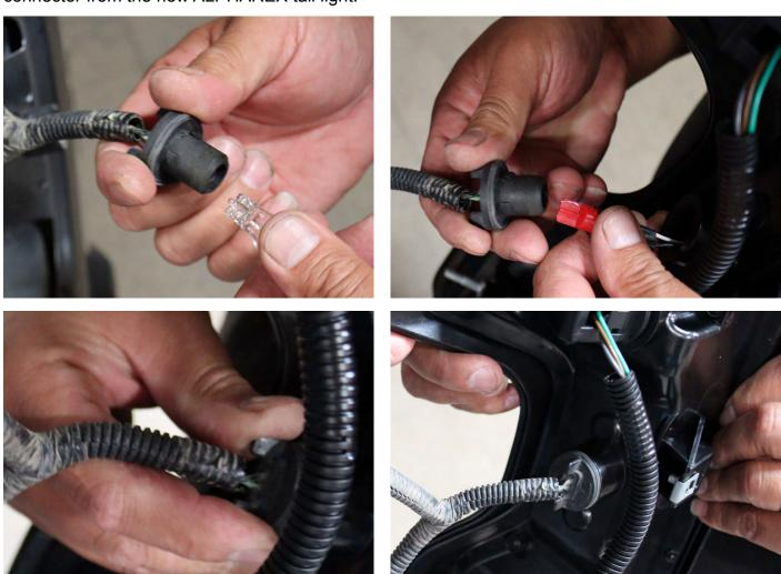
Lastly, plug the vehicle's tail light socket to new ALPHARE tail light connector.
