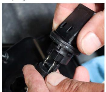
Twist and secure the socket tightly
