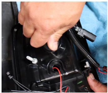
Twist and secure the socket tightly
