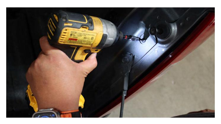
Remove the top and bottom T15 screws from each side of the tail lights.
