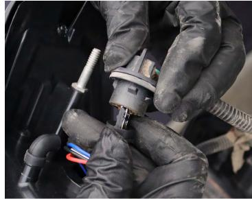
Twist and lock each of the sockets into the new ALPHAREX tail light.
