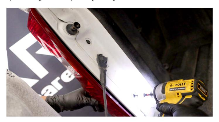
Remove the top and bottom T15 screws from each side of the tail lights.
