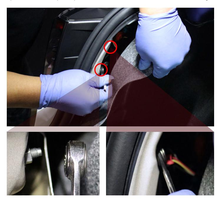
Disconnect the tail light wires.
