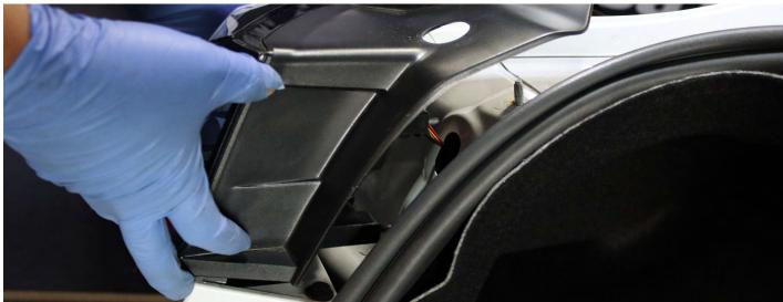
Completely detach and remove the outer section of the tail light.
