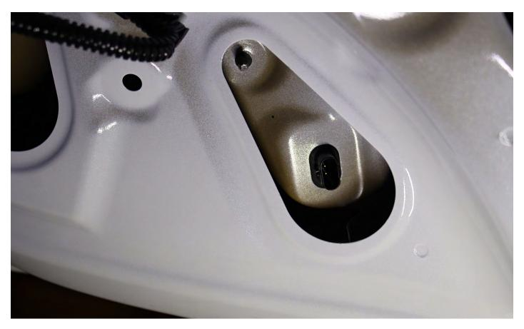
Using a plastic plier, delicately pull and detach the inner section of the tail lights.
