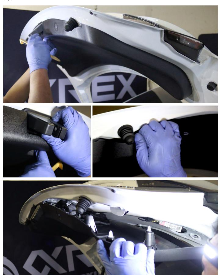
If your Tesla Model 3 is equipped with a power liftgate trunk, ensure to unplug the wire while removing the trunk panel.
