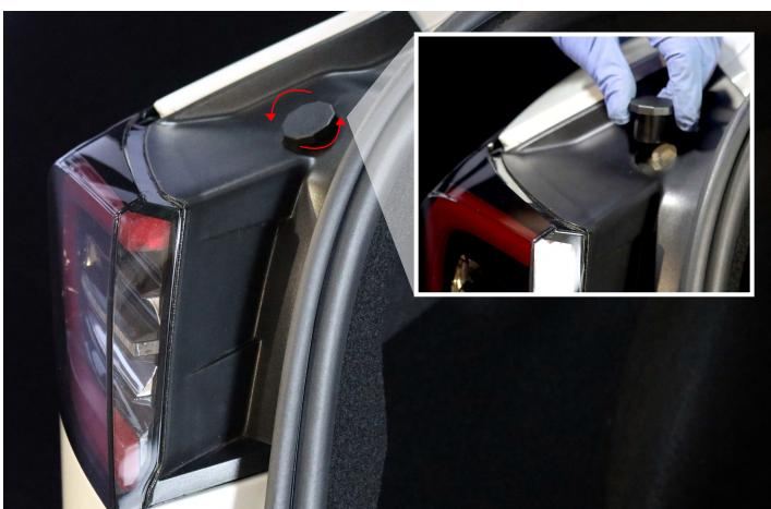
Open the side of the carpet and proceed to remove the two 8mm nuts from the back of the tail light.
