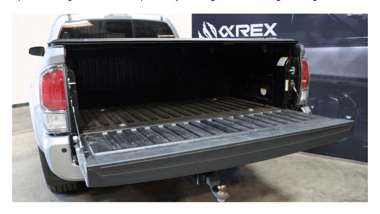
Take out the top and bottom 10mm bolts from each side of the tail lights.
