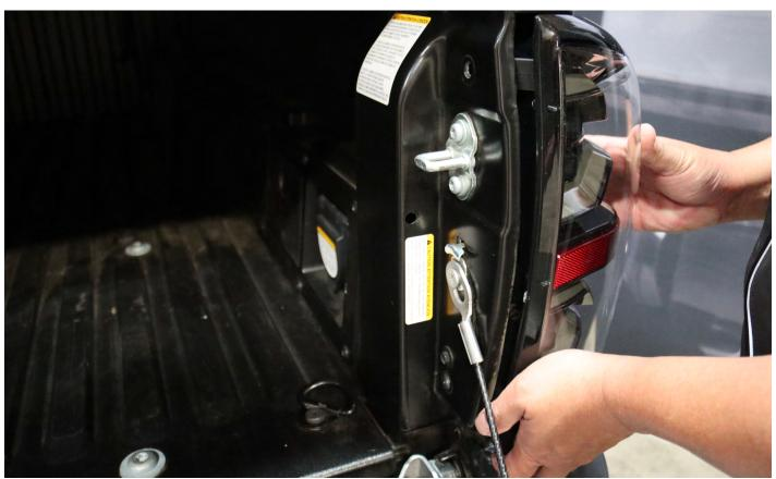
Utilize a ratchet to tighten the 2  $\times$  10mm bolts on each side. Note: When using a power wrench, ensure not to overtighten the bolts.
