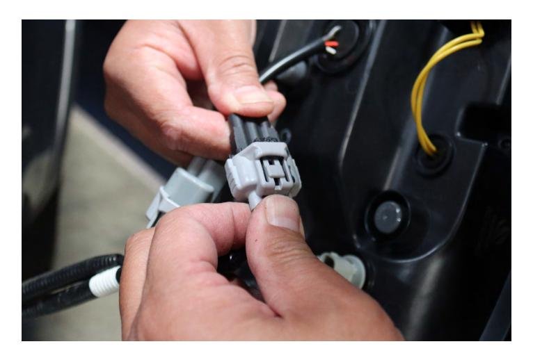
After plugging the sockets into the new ALPHAREX tail lights, proceed to reverse the removal process to install the new tail lights into the vehicle.
