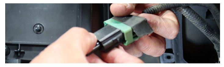
Ensure the connections are correct. NO DIELECTRIC GREASE should be used.
