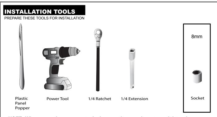
NOTE: Whenever using a power tool, please make sure do not overtighten the screws.
