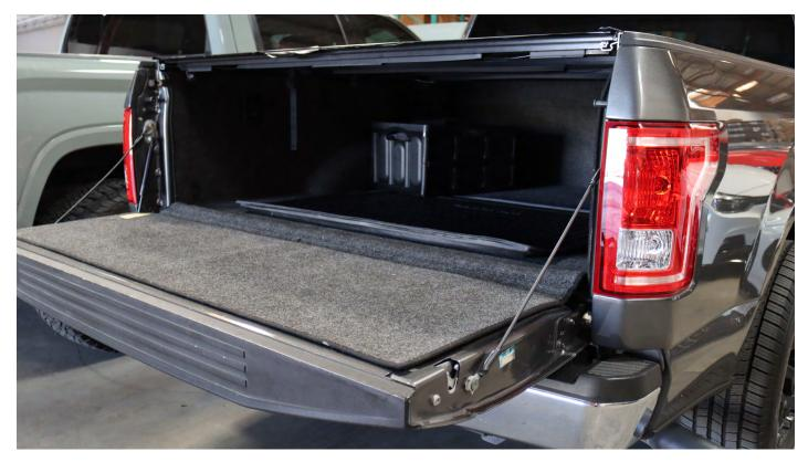
Remove the top and bottom 8mm bolts from each side of the tail lights. NOTE: When using a power wrench, ensure not to overtighten the bolts.
