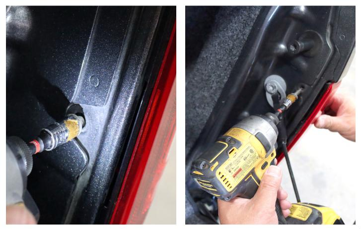
Carefully pull the tail light outward to remove it.
