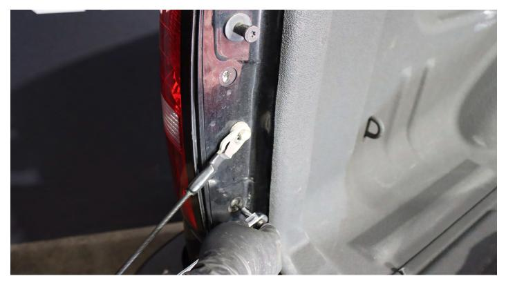
Take out the top and bottom T15 screws from each side of the tail lights.
