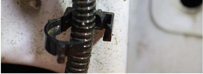
There are (2) cable clips securing the wiring for the driver's side tail light and (4) cable clips securing the wiring for the passenger's side tail light.
