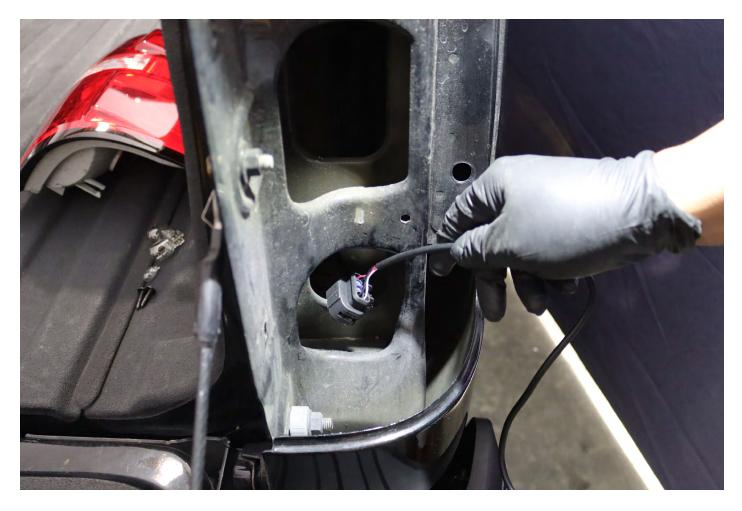
Route the tail light wiring into the truck as shown in the illustration, securing each section using the factory plastic connector mounts. **DO NOT USE DIELECTRIC GREASE!**
