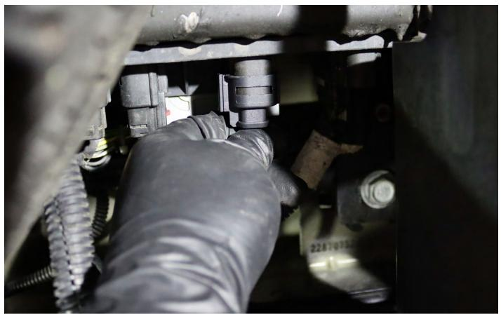
Plug in the wiring sockets as shown in the picture below. DO NOT USE DIELECTRIC GREASE!
