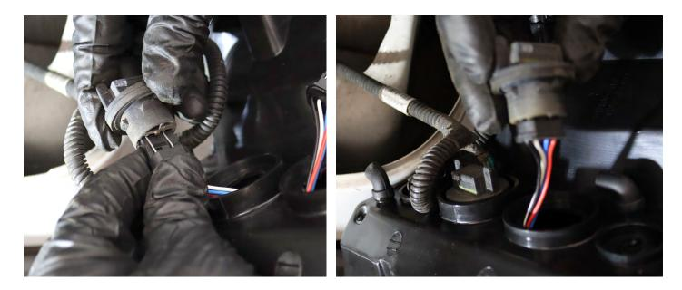
Twist and lock each of the sockets into the new ALPHAREX tail light, ensuring they are tightened and secured. **DO NOT USE DIELECTRIC GREASE!** Follow the same steps for the other tail light.
