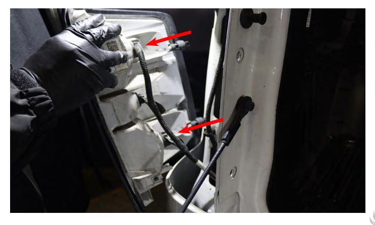
Disconnect the reverse light socket and keep the light bulb for future reinstallation.
