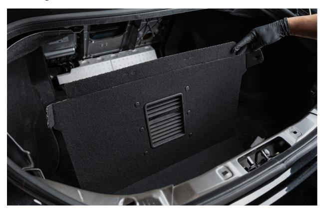
1.6 - With the rear panel removed, you'll now have access to remove the outer trunk panels as well.
