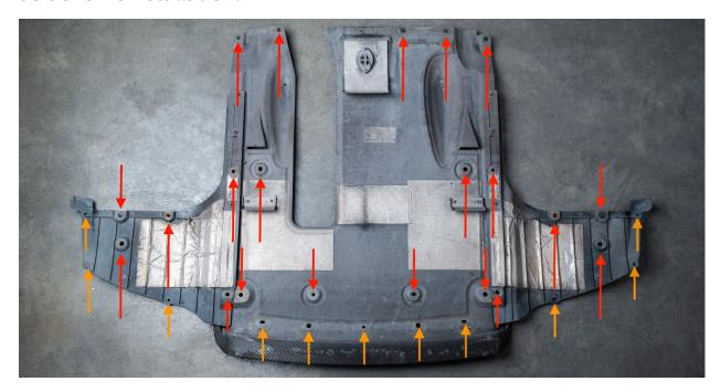
1.14 - Begin by removing the five clips located along the rear center section of the diffuser and the six towards the outer edges.
