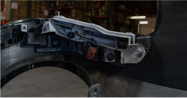
1.25 - With everything disconnected and the bumper out of the way, the OEM tail light can now be fully removed from the vehicle. You're now ready to move forward with installing your new Alpharex tail lights.
