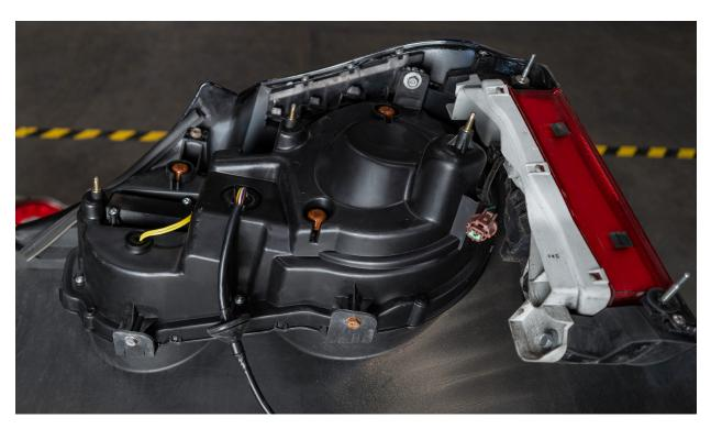
2.2 - To complete the installation, begin reinstalling all previously removed components in reverse order. Before fully reassembling the vehicle, we recommend testing the new Alpharex tail light to ensure all functions—brake, turn signal, reverse, and running lights—are working correctly. This will help avoid the need to disassemble again if adjustments are needed.
