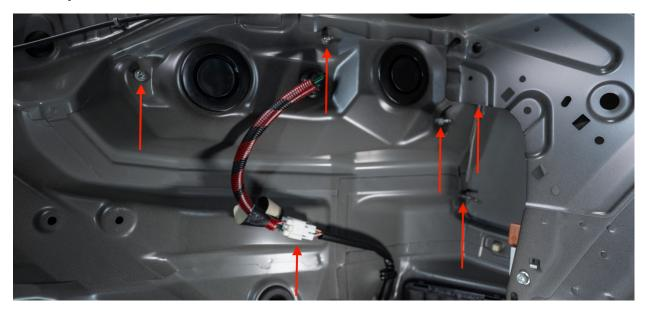
1.8 - Note: One of the five 8 mm nuts is located behind the panel and will require reaching behind the trunk sheet metal to access it.
