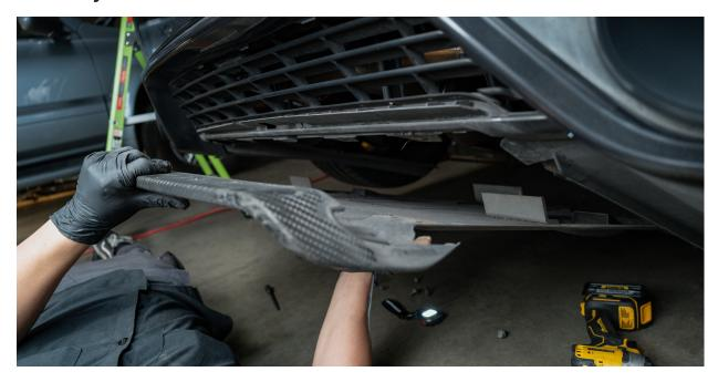
1.18 - With the diffuser removed, you'll now have access to a hidden bracket securing the bumper. Locate a single 10 mm nut positioned toward the outer edge of the bumper. Remove this nut to release the bracket.
