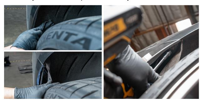
1.20 - You can now begin removing the bumper. Start at the outer edges and gently pull them back to release the bumper from the body. As you work your way inward, use a flathead screwdriver or trim tool to carefully release the clips securing the bumper in place. Take your time and be gentle to avoid damaging any mounting tabs or paint.
