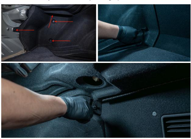
1.4 - Now proceed to remove the top panel. This panel is secured with three clips that will need to be removed.
