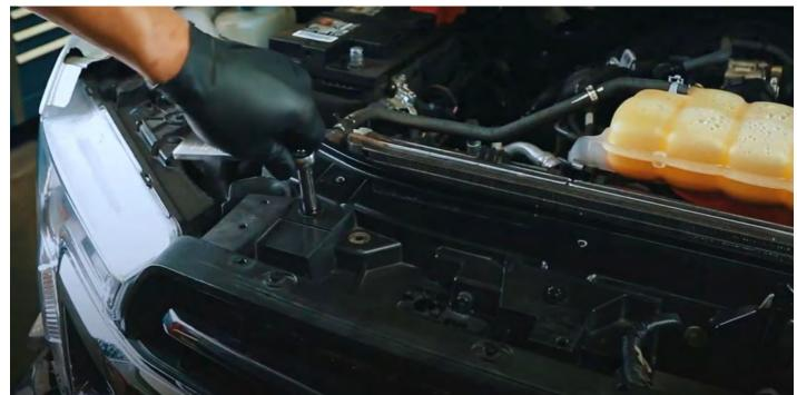
Unscrew the 8mm bolt located beneath each headlight and proceed with their removal.
