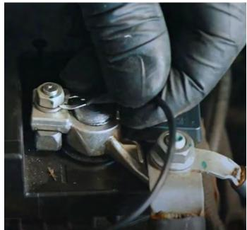
Use zip ties to secure and fasten the yellow connection to the daytime running lights harness, ensuring a stable and tidy arrangement.
