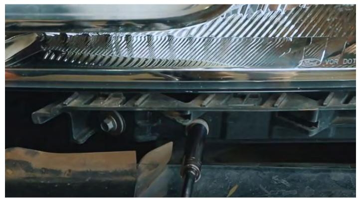
Additionally, there is one 10mm bolt situated behind the fender flare that needs to be removed to detach the headlight.
