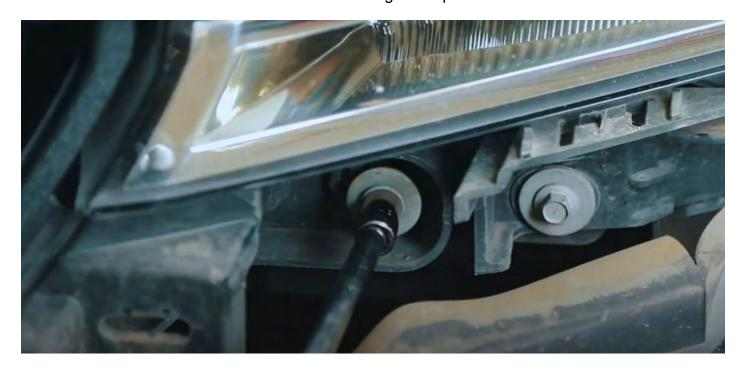
Detach the plastic clips that secure the light wiring.
