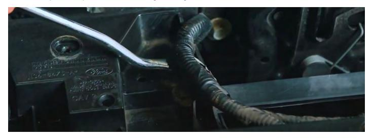
Disconnect the two connections for the active grille located at the top of the radiator area.
