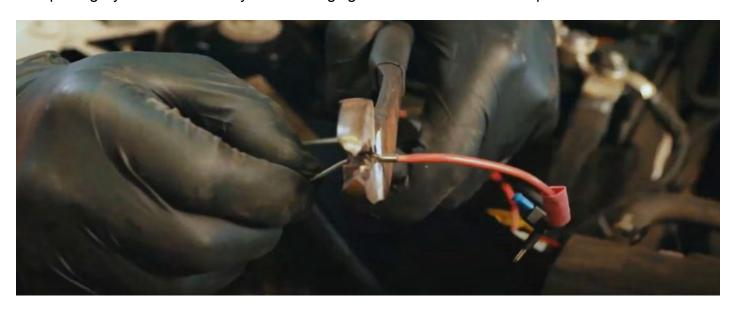
Proceed to the fuse box and tap into either fuse number 36 or fuse number 10 using the fuse tap.
