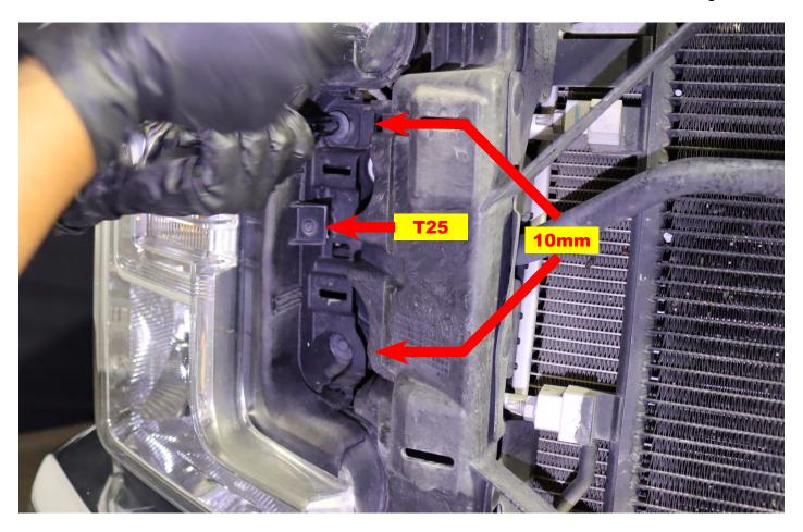
Utilize an extension to assist in removing the 10mm bolt from the side of the headlight, located inside the front fender and bumper mounts. Repeat these steps for the other side of the headlight.
