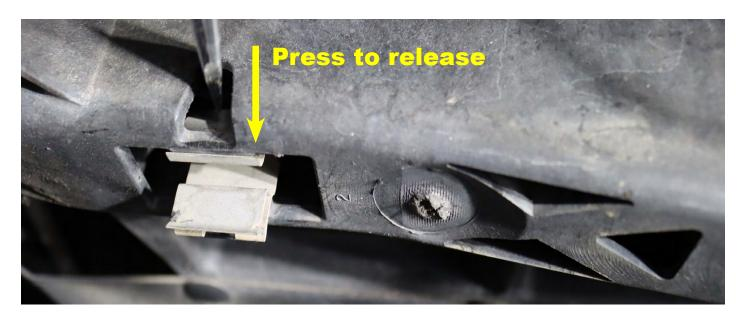
Subsequently, gently pull the grille outward towards you to disengage it from all the mounting points and remove the front grille. If your truck is equipped with a Front View Camera Washer, ensure to unplug the nozzle's tube and the wiring before removing the grille.
