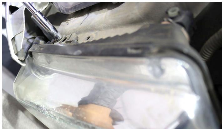
Proceed to remove the two 10mm bolts and one T25 bolt located on the side of the headlight.
