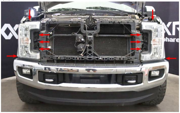
Utilize a ratchet to unscrew the top 10mm bolts securing the headlight.
