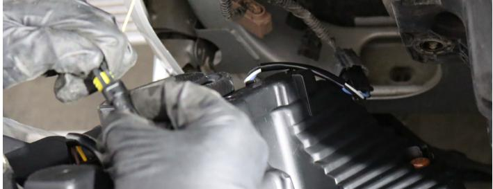
Secure the harness to the daytime running light connection on the back of the headlight.
