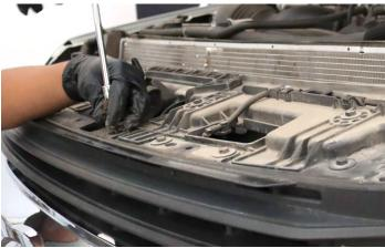
Next, employ a flat screwdriver to assist in releasing the (4) grille molding clips located at the bottom of the grille.
