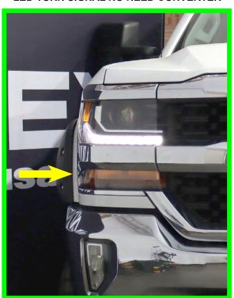
IF YOUR VEHICLE IS EQUIPPED WITH LED TURN SIGNAL A CONVERTER IS NEEDED
