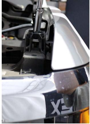
To access the headlight bolt from the inner bumper, first, remove the 2 X T15 screws from the wheelwell.
