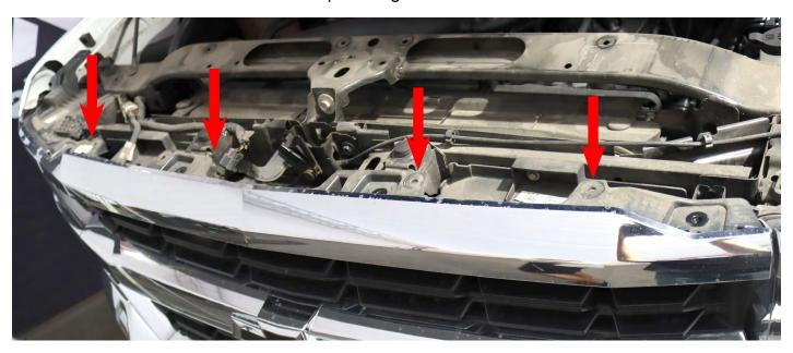
Subsequently, carefully pull the grille towards you to release it from the 6 insert mounts. Set it aside for later reinstallation.
