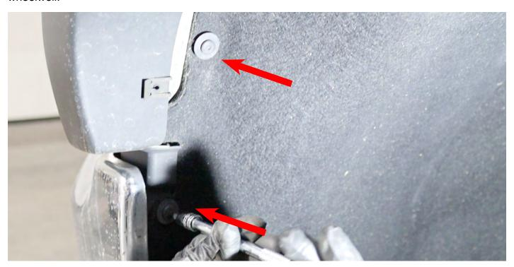
Subsequently, use a panel popper to widely open the guard cover, providing access to the headlight's bolt. Utilize a ratchet and extension socket to help remove the 10mm bolt. Repeat the same steps for the other side of the headlight.
