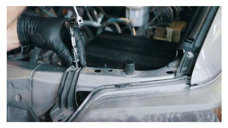
Lift up on the two top arms and remove the headlight from the truck. *Please follow the same procedure for the other side.*
