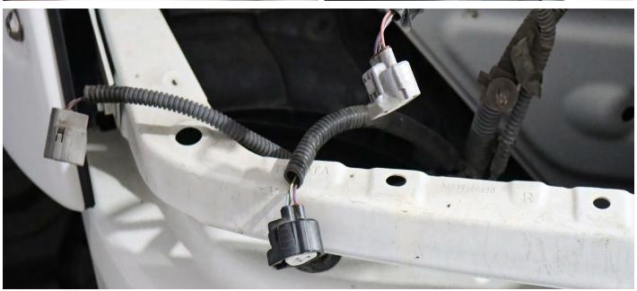
Transfer the turn signal bulb into the new ALPHAREX headlight.
