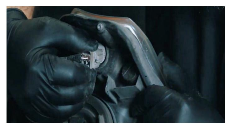
Use the panel popper to release the wiring harness from the headlight.
