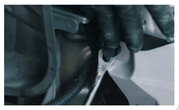
Once the bolts and clips are removed, carefully remove the trim piece and set it aside to be reinstalled later.
