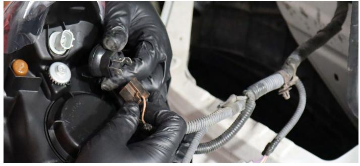
Attach the harness to the daytime running light connection on the back of the headlight.
