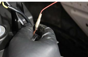
Reattach the headlight wiring harness on to the ALPHAREX headlight. **DO NOT USE DIELECTRIC GREASE!**
