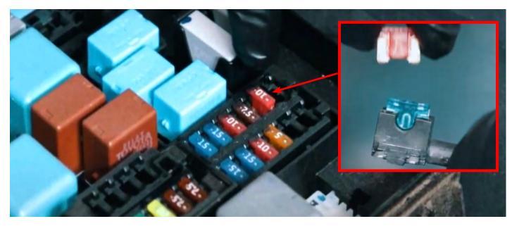
Crimp the gray wire from the harness to the fuse tap and reinstall the fuse box cover.
