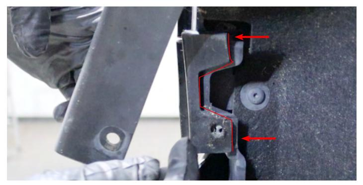
Carefully pull the edge of the trim outward to release it from the mounting.
