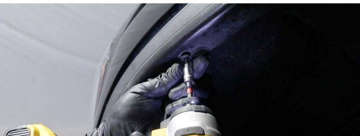
Utilize the panel popper to gently lift up the fender guard partially from the mounting spots and release it.
