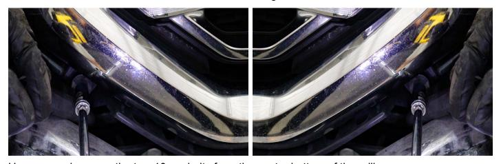
Unscrew and remove the two 10mm bolts from the center bottom of the grille.
