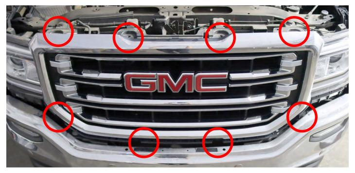
Take out the 10mm bolt from the bottom corner of the grille, one on each side.
