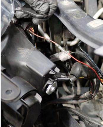
Finish the installation by securing the headlights to the truck. Reverse the headlight removal process to complete the installation.
