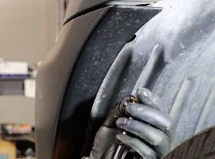
Lift the edges of the bumper to release it, and carefully pull it outward.
