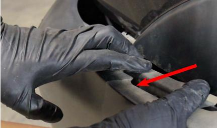
Use a panel popper to remove the two plastic retainers from the front bumper.
