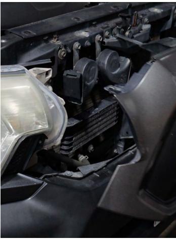
Next, remove the plastic trims to gain access to the headlight bolts.
