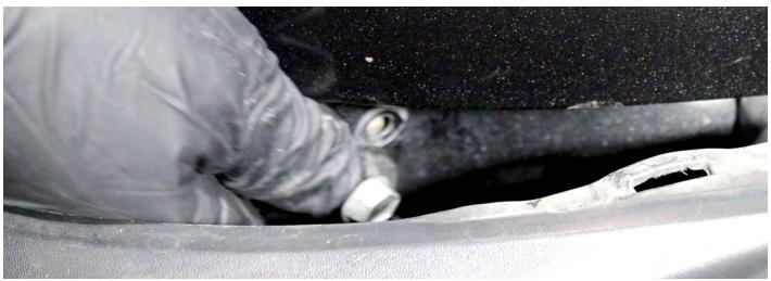
Remove the two 10mm bolts from the top of the headlight.
