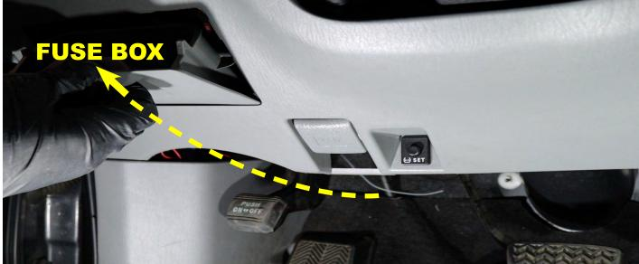
Open the fuse box under the driver's side dash and tap into the IGN (ignition) fuse.
