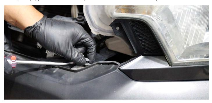
Loosen and release the bumper until you have enough space to reach the bottom of the headlight's bolt. Repeat the same steps for the other side of the bumper.
