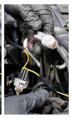
Attach the harness to the daytime running light connection on the back of the headlight. Repeat the same steps for the other side of the headlight.
