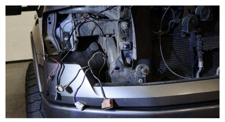
Once you've successfully routed the necessary wire harness(es), you are now ready to proceed with the installation of the new ALPHAREX headlights.
