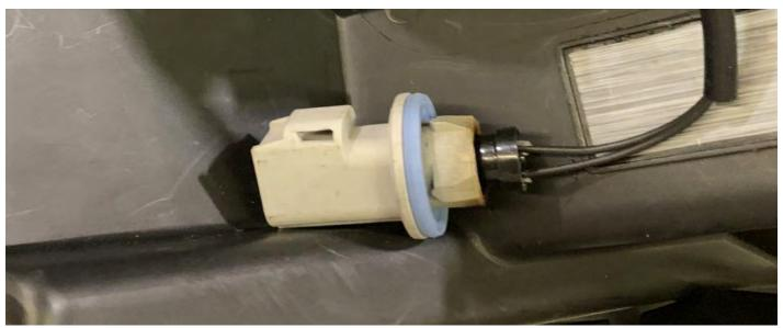
Connect one end of the turn signal split connection to the new headlight turn signal socket. Repeat the same procedure for the other headlight.
