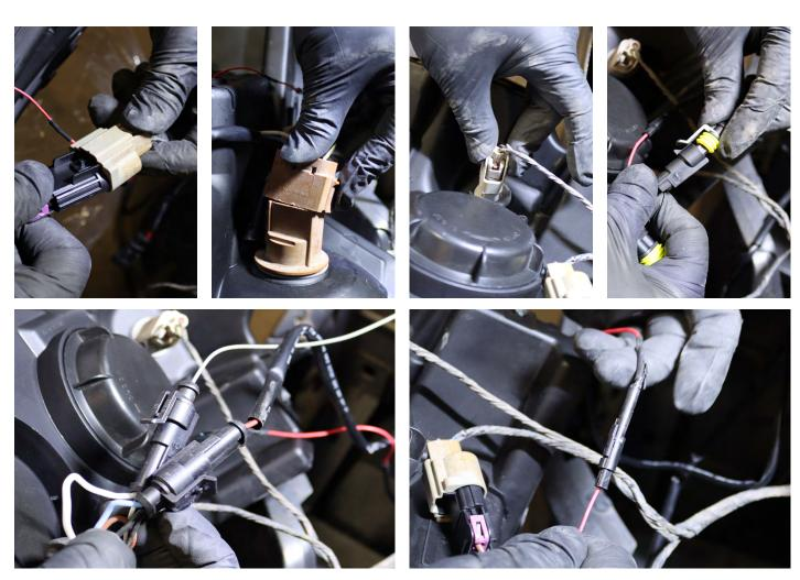
Ensure that all the sockets are firmly and securely connected to the new headlights before proceeding with the installation into the vehicle. Repeat the same process for the other side of the headlight.
