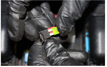
Once the fuse box cover is closed, route the DRL harness wire towards the driver side of the headlight location.
