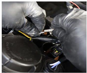
Complete the installation process by securely attaching the headlight to the truck. Repeat the previous steps for the opposite side headlight installation to ensure consistency on both sides.
