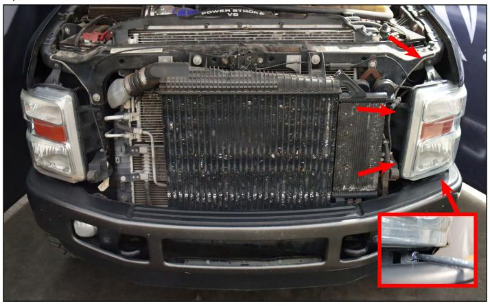
After removing the bolts, carefully pull the headlight forward and unplug the light sockets to facilitate headlight removal. Repeat the same steps for the other side.
