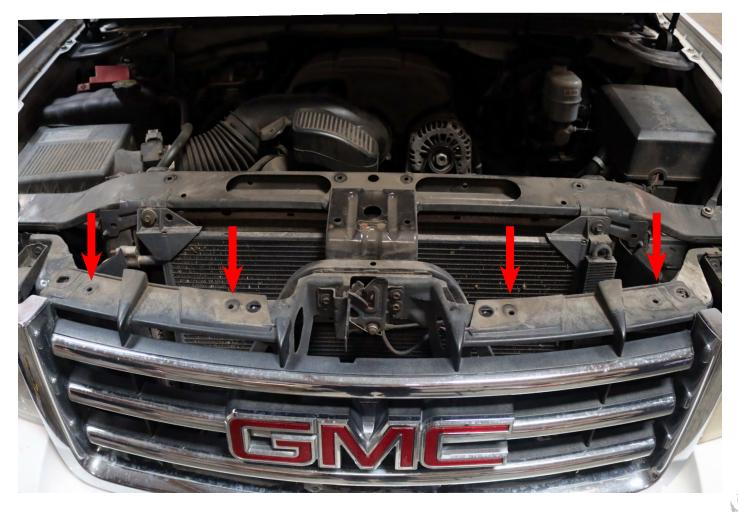
Afterward, use pliers to compress the four metal clips and pull outward to release the grille.
